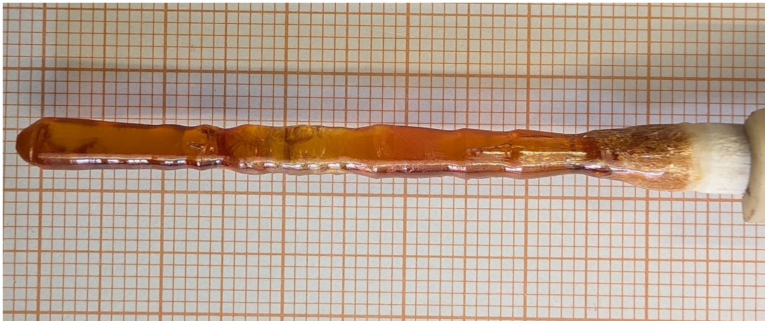
Fig. 1. The crystal grown by optical floating zone method.
